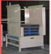
Pallet dispensers and pallet conveying for auto bag removal
