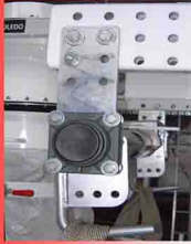
Drive-off type loop support arms complete with adjustment holes to accommodate different bulk bags
