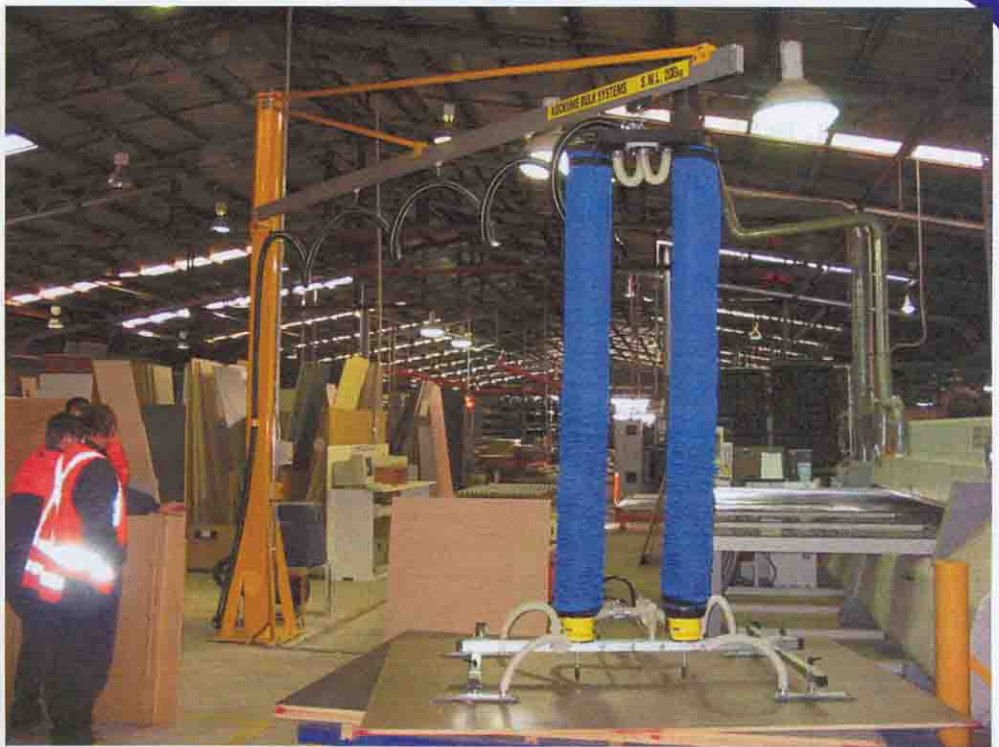
Vaculift Lifting System with column & swing arm bringing stock to the machine centre.
