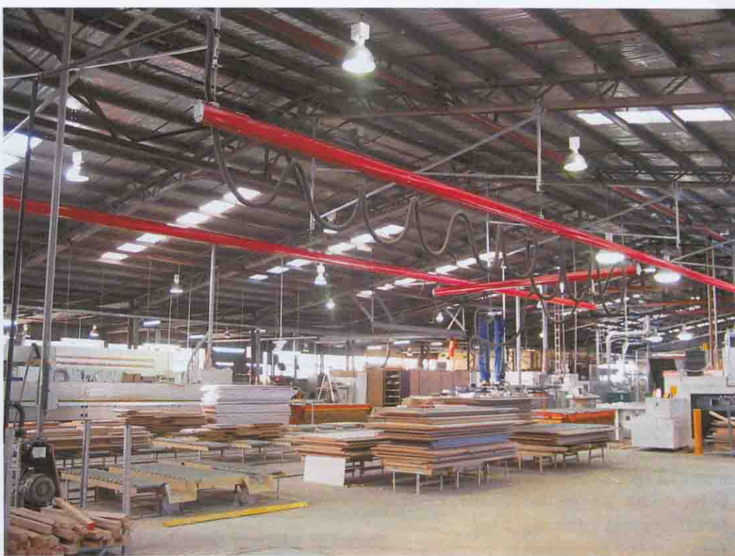
General view of a typical 20m track, with a Vaculift unit on the bridge
