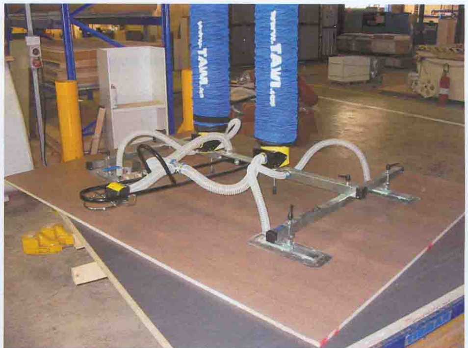
Wide spread of lifting feet for stability.
