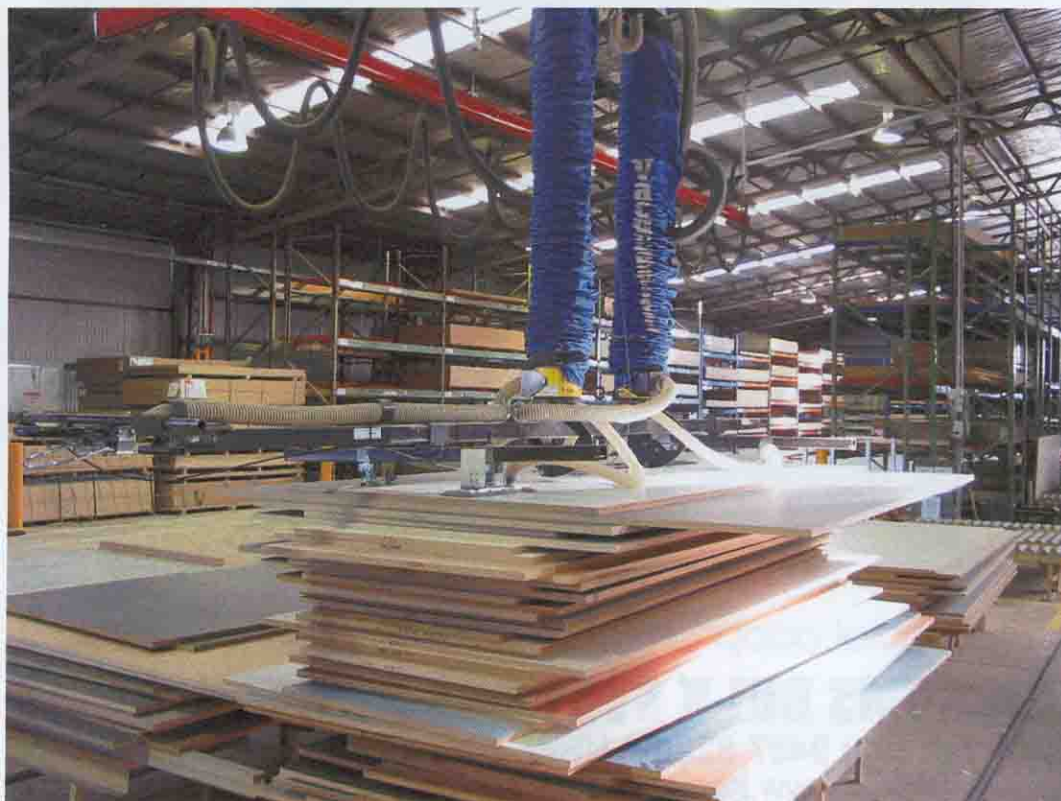
View of lift tubes, lifting heads, feet and control handle.
